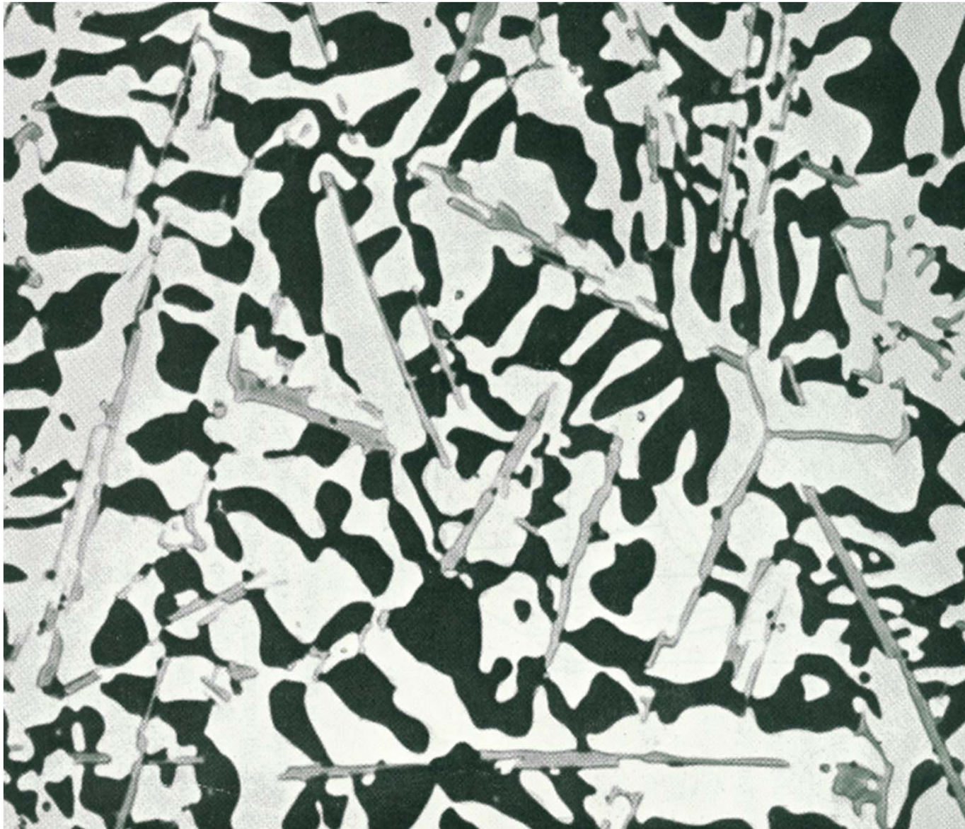
Microstructure of the ternary eutectic in the Al-Cu-Si system. 32 \alpha light, \theta dark, Si grey, (x 900)
