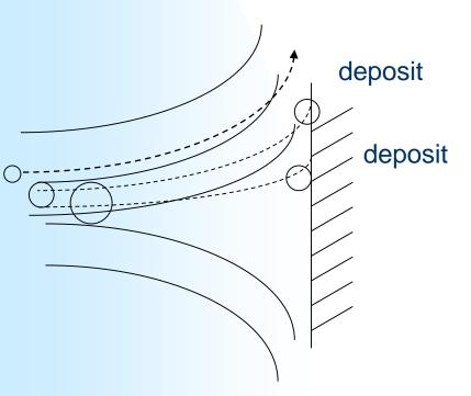
So, it is very difficult to collect small particles by utilizing inertial force.
