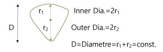
Causes: Jaws chucking, or centerless grinding
