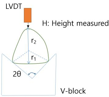
$H_2=r_2+r_2/\sin\theta$ : measured at 2 position
