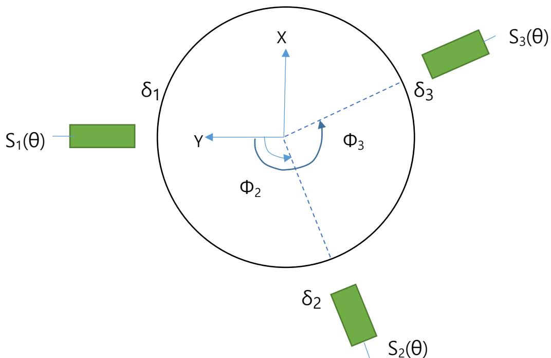
$\delta_1, \delta_2, \delta_3$ : stand-off distances from each sensor when disc rotates  $\theta$  angle
