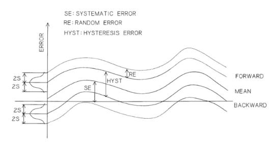
Calibration curve for the rotary or indexing table
