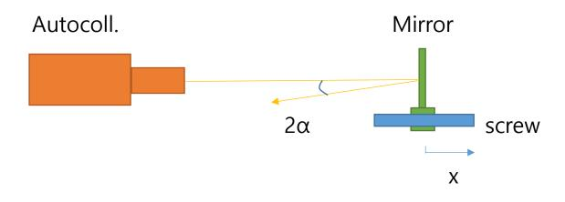
The pitch angle, and yaw angle can be measured by the autocollimator, but not for the roll measurement.
