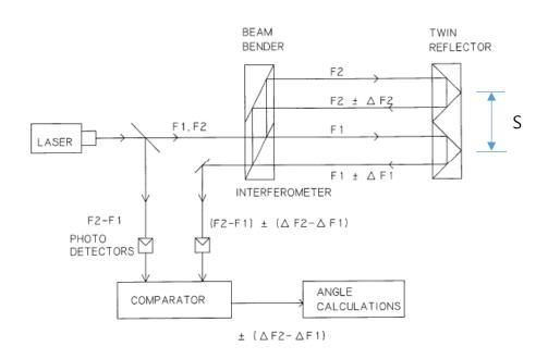
FIG.7.7 PRINCIPLE OF ANGLE MEASUREMENT WITH LASER INTERFEROMETER
