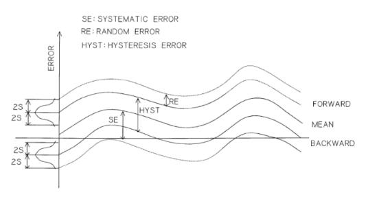
With the laser angular optics and the autocollimator, the measurable error components are;
