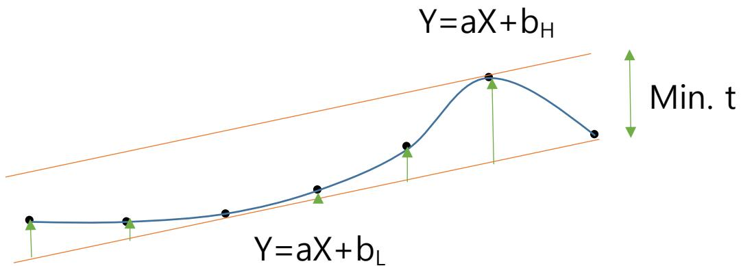
Two parallel lines containing the measured data, and the minimum distance  $t=b_H-b_L$  (that is, minimum separation, or minimum zone).
