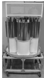
High sensitivity directional radiation detection system (rotating) by SNL
