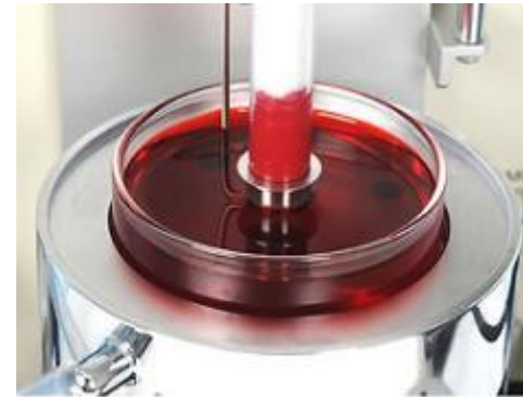
Appearance and penetration of powder packed column
