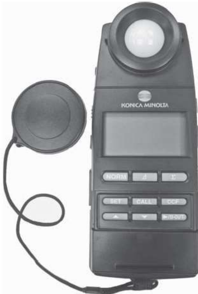
Fig. 6.8 Electronic, digital, color-corrected, and cosine-corrected illuminance meter from Konica-Minolta.
