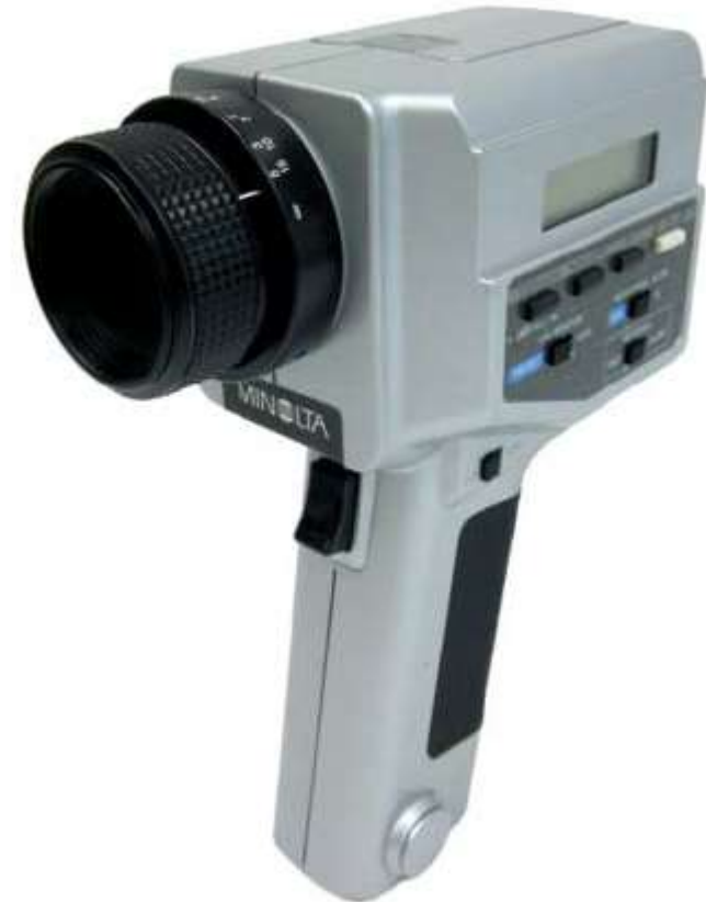
Fig. 6.10 Direct-reading, narrow-angle, spot-type luminance meter has an acceptance angle of 1^\circ , a range of 0.001 to 299,000 \text{cd}/\text{m}^2 ( 0.001 to 87,000 \text{fL} ), a variable response speed to permit measurement of flickering sources, and a comparison mode that permits direct luminance comparison of two sources. Results are displayed digitally.
