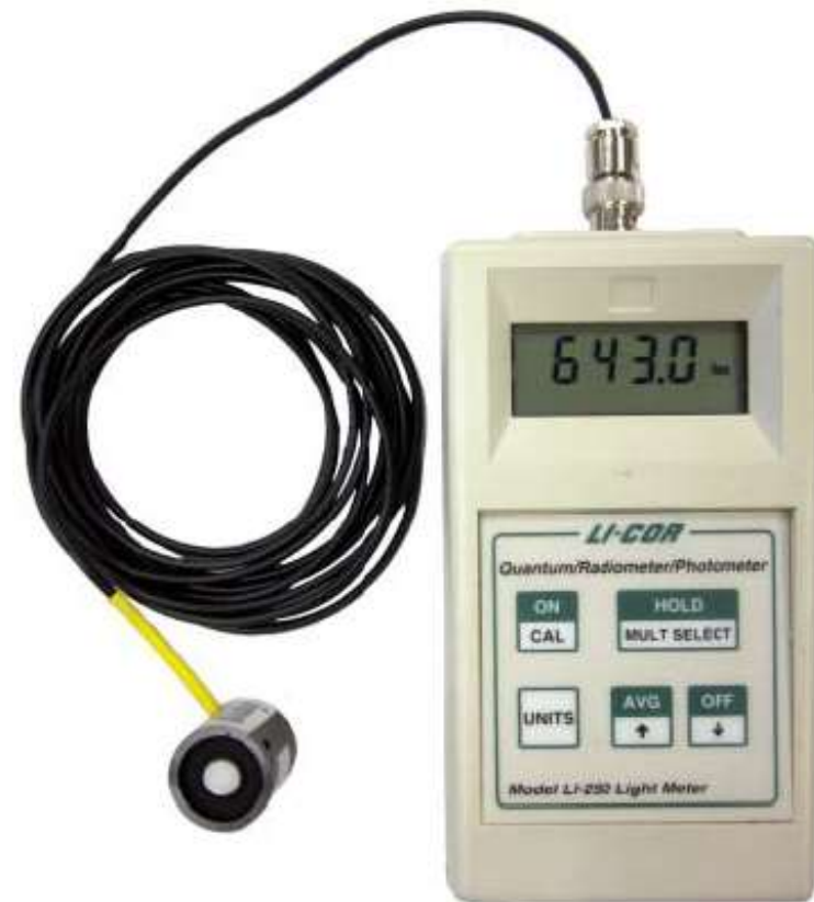
Fig. 6.9 Digital meter (from Li-Cor) has a variety of sensors that measure illuminance, solar irradiance, or photosynthetic radiation. Due to its small size, the illuminance sensor can be easily used for architectural model measurements.
