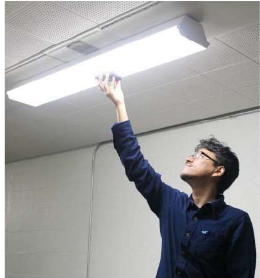
Fig. 6.11 When the cell of a direct-reading illuminance meter is held in contact with a luminous source, the surface luminance can be read directly or calculated.
