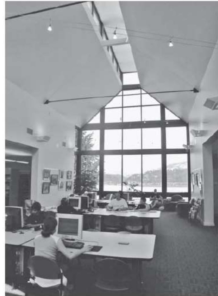
Fig. 1.18 Seek common solutions. The "atrium" of the Hood River County Library, Hood River, Oregon, provides a central hub for the library, daylighting, views (spectacular), and stack ventilation. (© Alison Kwok; all rights reserved.)
