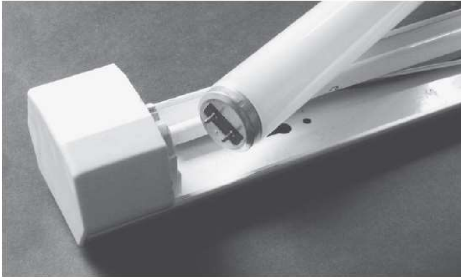
Fig. 15.10 Rapid-start fluorescent lamps have two pins that slide against two contact points in an electrical circuit. The ballast constantly channels current through both electrodes, creating a charge difference between the two electrodes and establishing a voltage across the tube. (Photo by Jonathan Meendering; © Alison Kwok; all rights reserved.)
