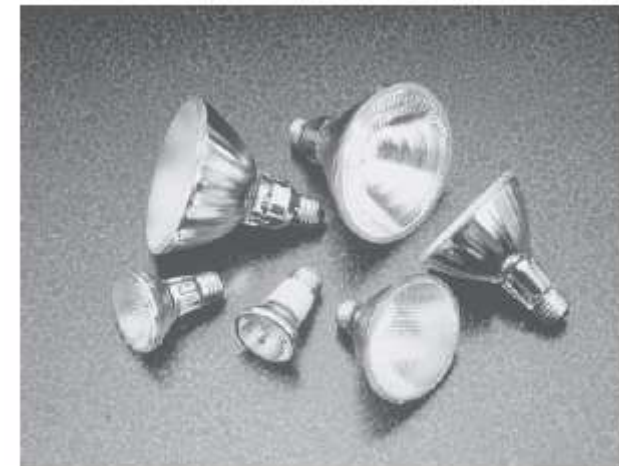
Fig. 15.5 PAR halogen lamps with standard medium screw bases in sizes PAR 16, 20, 30, and 38 with a short or elongated lamp neck. Lamp wattages range from 45 to 90 W. (Courtesy of Philips Lighting Co.)
