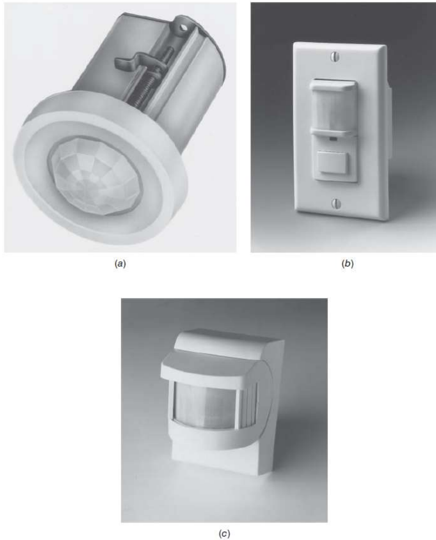
Fig. 15.52 Passive infrared (PIR) occupancy sensors. All sensors can be equipped with an adjustable override to prevent turning on lighting when ambient light is sufficient. All units have adjustable delayed-off timing and a flashing LED that indicates sensor operation. (a) Flush-mounted ceiling unit. The 360° circular pattern of the lens indicates omnidirectional coverage. The unit is approximately 4 in. (100 mm) in diameter. (b) Flush-mounted combination wall switch and PIR occupancy sensor. Operation of the switch overrides the sensor function. (c) Surface-mounted wall PIR occupancy sensor. The semicircular shape of the lens indicates wide horizontal coverage. (Photos courtesy of Leviton Manufacturing Co.)
