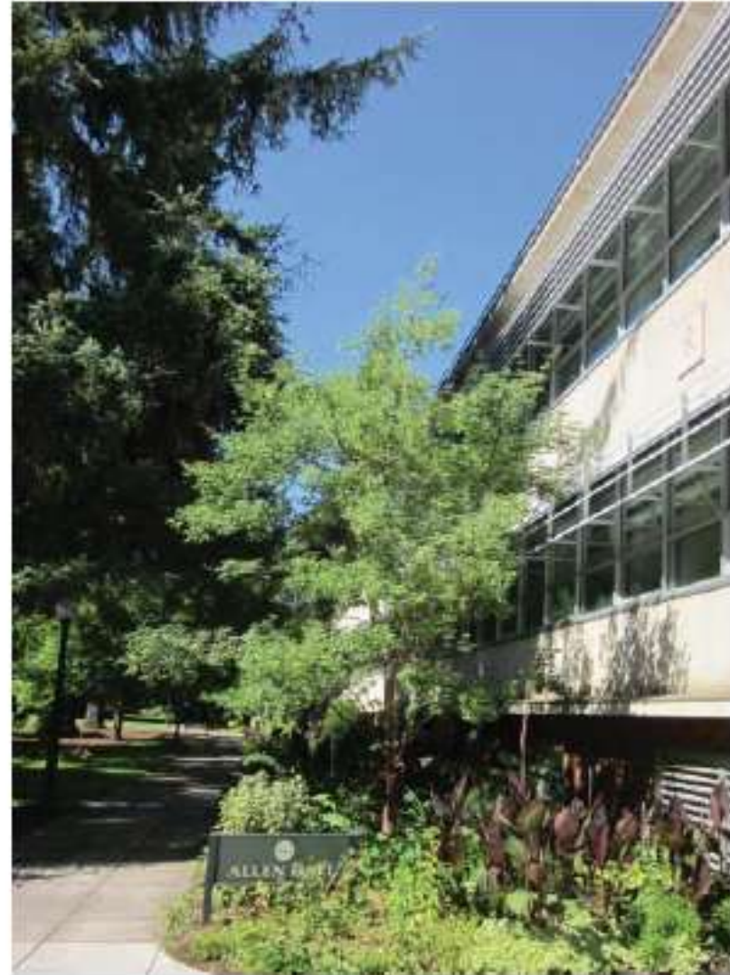
Fig. 3.41 A deciduous tree as a naturally "smart" shading device. (Courtesy Tyler Mavichien.)
