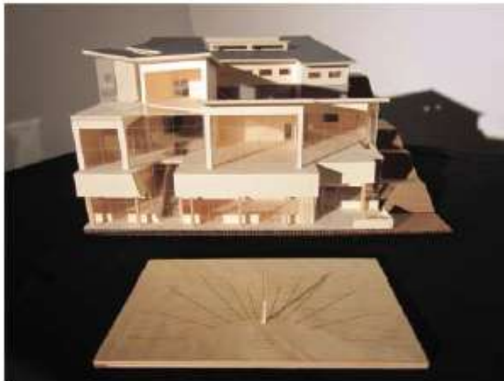
Fig. 3.16 A model of a small building with a glazed open-frame circulation space on the south side is observed at the sun's position at 3:00 p.m. on December 21 through the use of a sunpeg chart. (Photo by Tyler Mavichien; © Alison Kwok; all rights reserved.)
