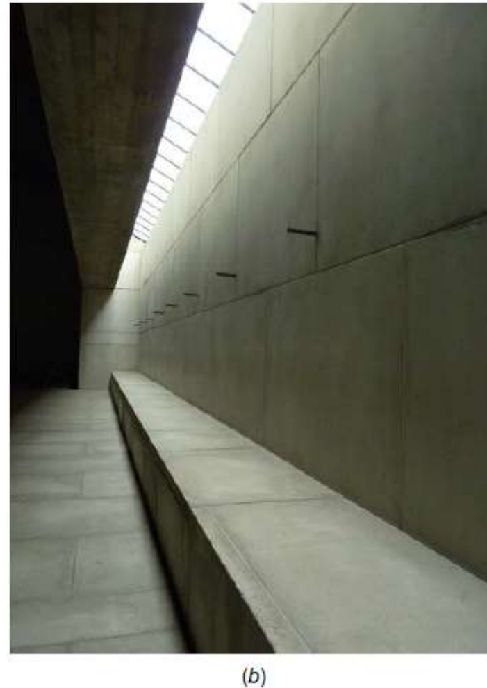
Fig. 10.16 (a) A skylight near a north wall provides reflecting surfaces for uniform light distribution and reduces the potential for glare. (b) The linear toplight enables light to wash an interior concrete wall at the Chapel of the Holy Cross, Turku, Finland (Pekka Pitkänen). (Drawing by Erik Winter; photo © Karen Tse; used with permission.)
