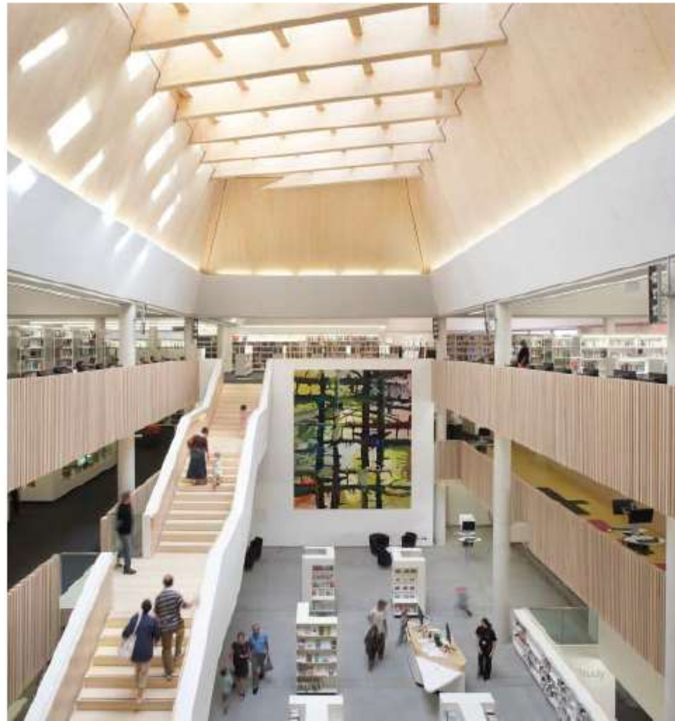
Fig. 10.54 Daylit atrium is controlled by the structural timber baffles; use of absorptive material around voids in the atrium provides a good acoustical environment. (Photo by Nick Hufton; © Hufton & Crow; used with permission.)
