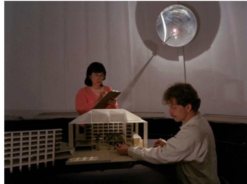
In the facility's interior, Osterhaus and Beltran conduct performance tests of a shading device for a hotel atrium using the sun simulator, upper right
