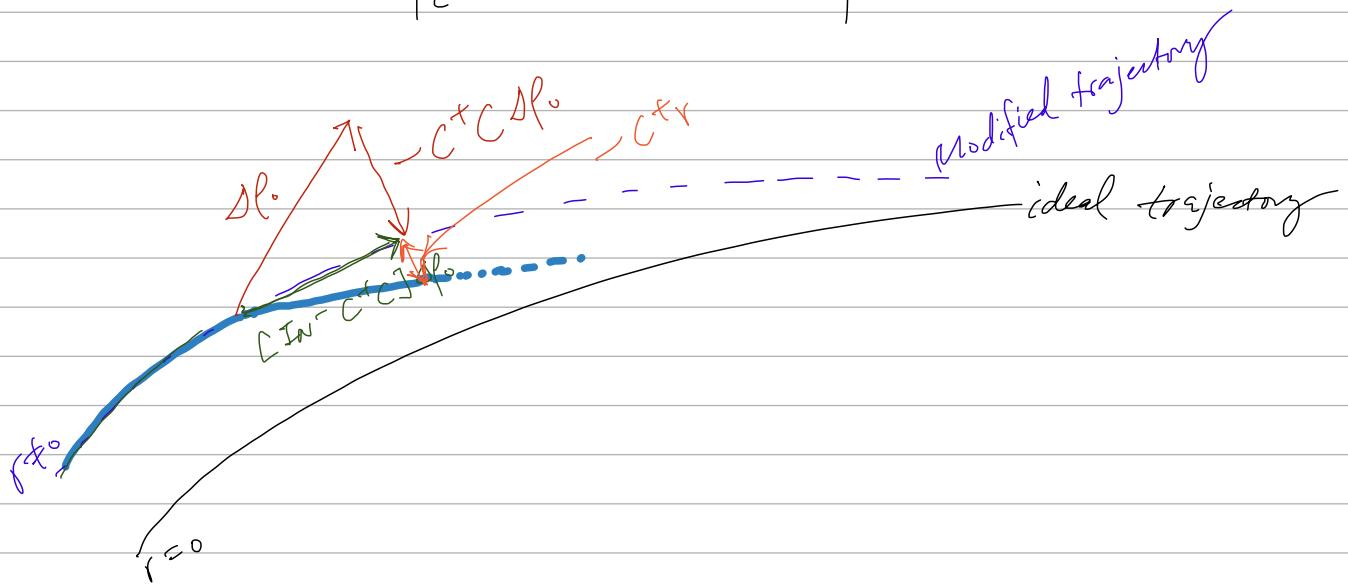
Euler integration results in accumulation of numerical errors
