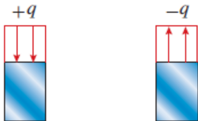
FIG. 9-4 Sign conventions for bending moment M , shear force V , and intensity q of distributed load
