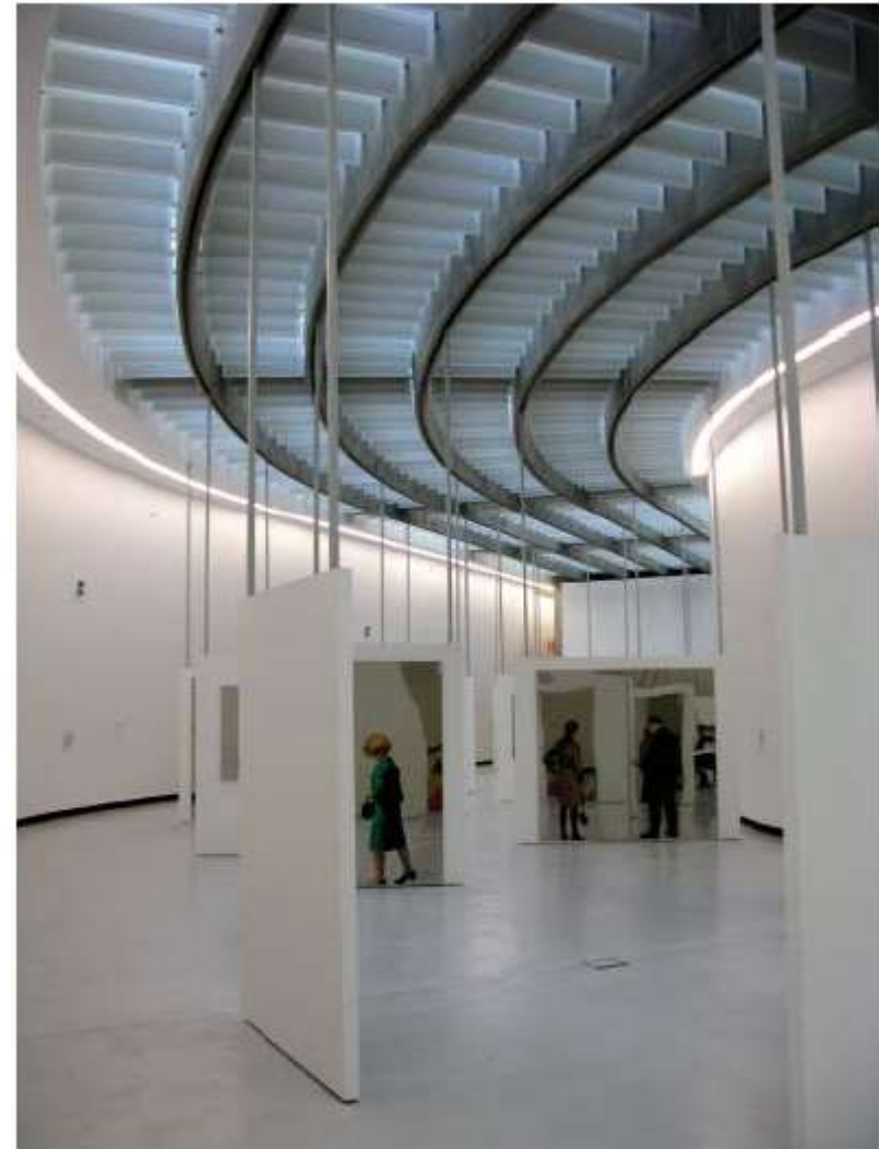
Fig. 16.37 Linear slot lighting emphasizes the curvilinear form of the gallery, further reinforcing a directional flow of traffic through the space. (© Donald Corner; used with permission.)
