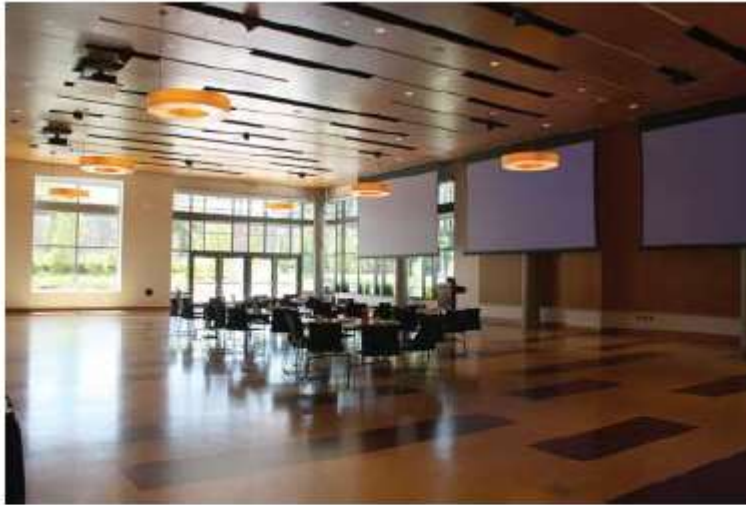
Fig. 17.10 Schools frequently utilize spaces for multiple functions. This space, typically used as a banquet room, doubles as an assembly room. High-intensity, recessed downlights in combination with large pendants provide sufficient light for both uses. (© Karen Tse; used with permission.)
