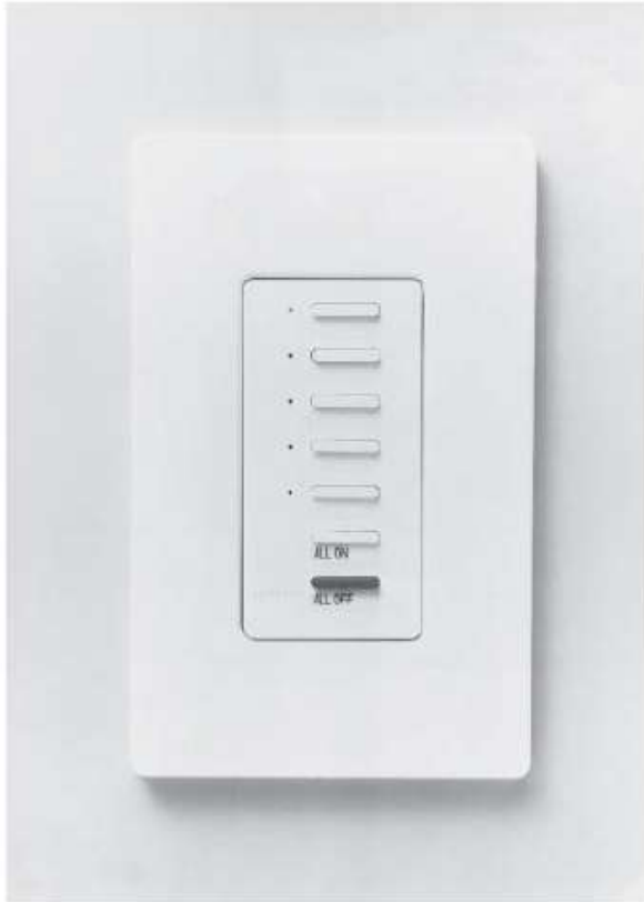
Fig. 17.5 Typical wall-mounted master station has five control buttons in addition to "All On" and "All Off" on every master. The control buttons can be arranged to control a single outlet or a group to establish lighting of a scene. Thus, the entry unit might have homecoming, extended absence, path lighting, nightlighting, and garage-lighting scenes, whereas the kitchen master may have lighting scenes for breakfast, dinner, formal and informal entertaining, and night. Each scene can be arranged to turn on, brighten or dim, and shut off selected lighting. (Courtesy of Lutron Electronics Co., Inc.)
