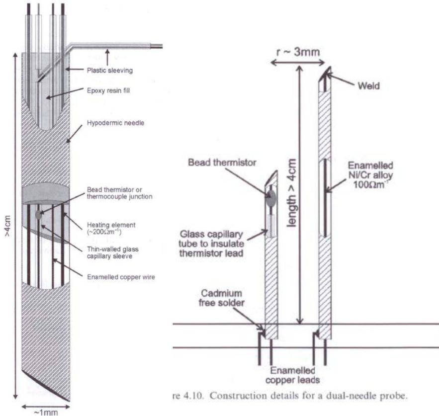
re 4.10. Construction details for a dual-needle probe.
