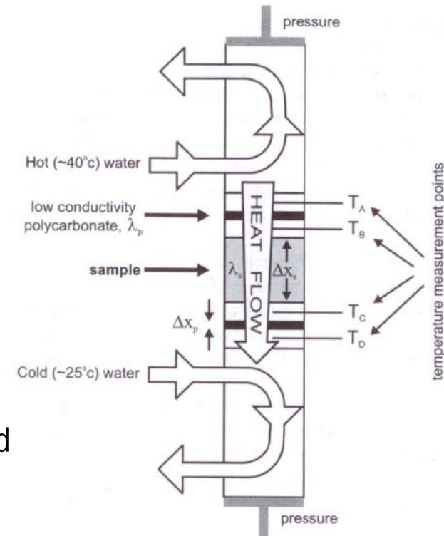
Figure 4.6. A typical divided-bar apparatus.
