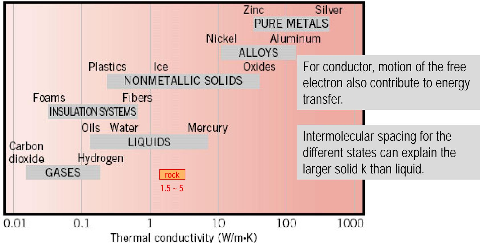
**FIGURE 2.4** Range of thermal conductivity for various states of matter at normal temperatures and pressure.
