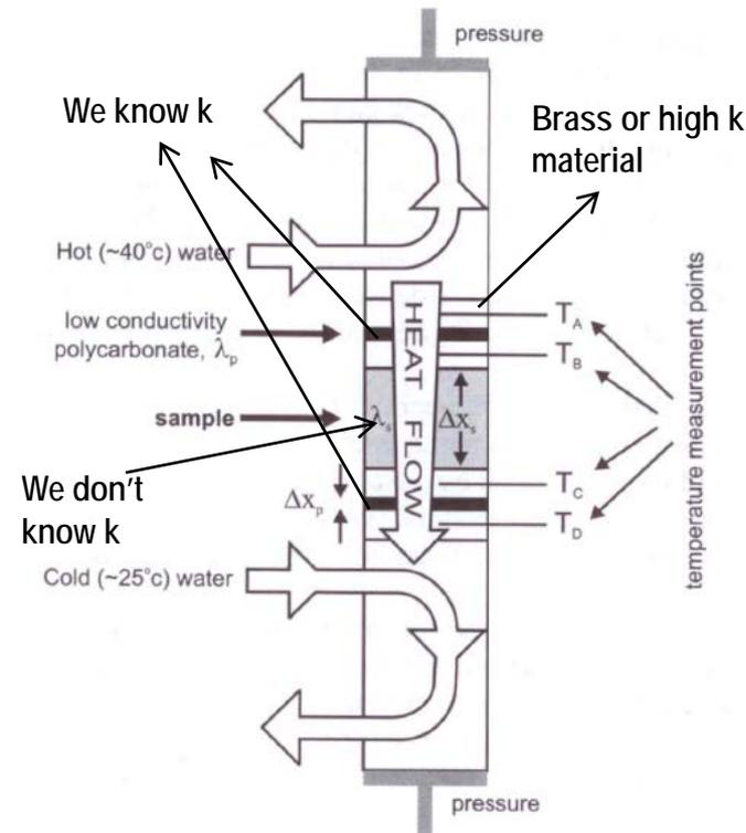
Figure 4.6. A typical divided-bar apparatus.
