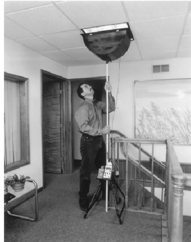
A fluxometer developed to measure a luminaire's available light in order to determine the benefits of periodic cleaning.
