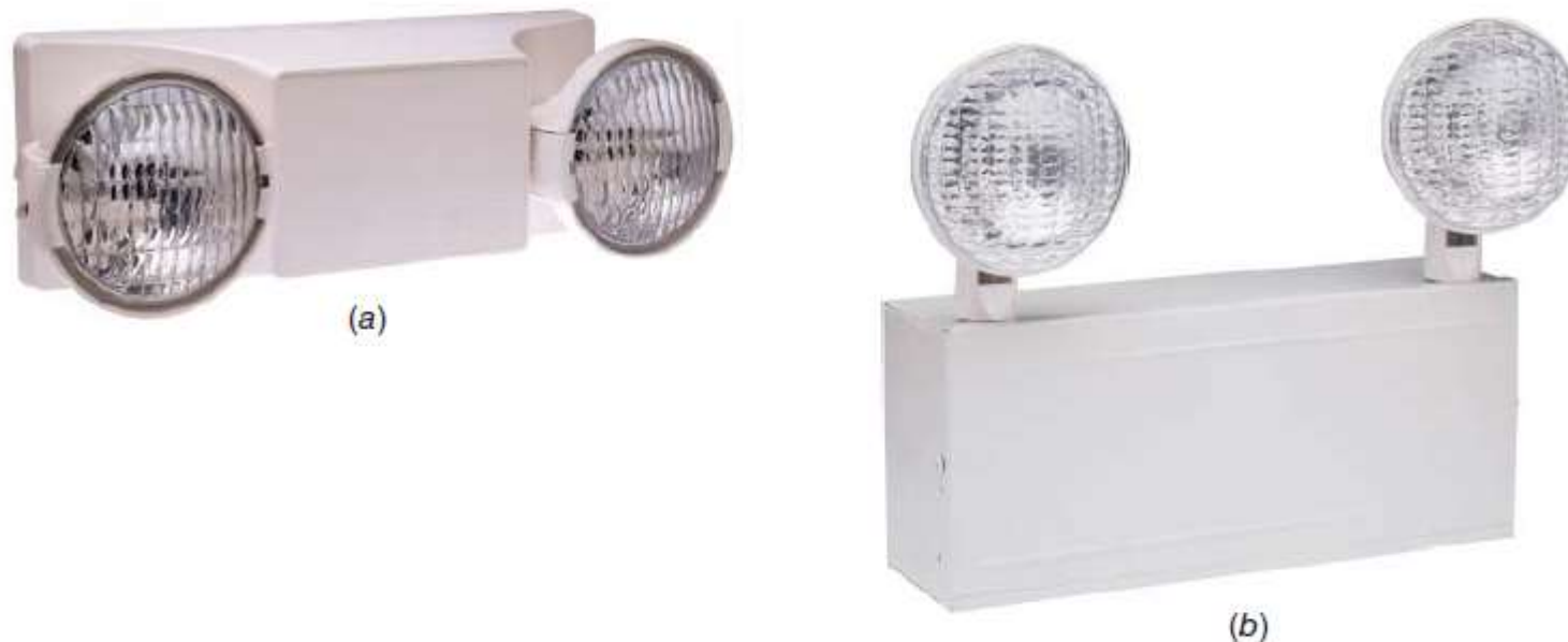
Fig. 17.25 Commercial emergency lighting units. (a) This decorative unit contains a sealed, maintenance-free lead-acid battery, an automatic charger, and an automatic low-battery-voltage disconnect. The battery is designed to supply a minimum of 90 minutes of operation of two fully adjustable 5.4-W sealed beam lamps. The unit measures 16.5 in. \times 5 in. \times 5 in. (419 mm \times 127 mm \times 127 mm). (b) Conventional design emergency unit contains a lead-acid or lead-calcium battery, which is housed with its required electronic control and safety equipment in a polycarbonate housing. The lamps are rated 7.2 W each. The entire unit measures approximately 15.75 in. \times 11.5 in. \times 4 in. (400 mm \times 292 mm \times 102 mm); exact dimensions vary with battery type, voltage, and capacity. (Courtesy of Dual-Lite, a division of Hubbell Lighting, Inc.)
