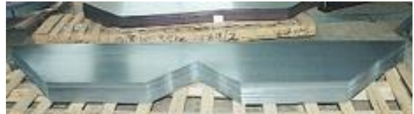
Stacked transformer core
