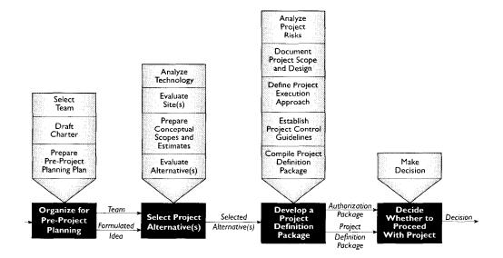
Figure I. I: Project Life Cycle Diagram
