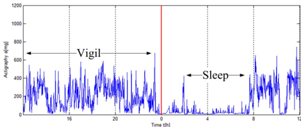
overall accelerometer activity (energy) during a vigilant phase vs. while sleeping.
