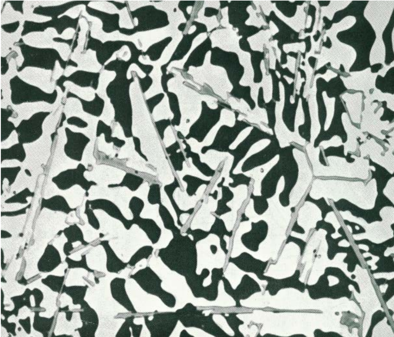
Microstructure of the ternary eutectic in the Al-Cu-Si system. \alpha light, \theta dark, Si grey, (x 900) 37
