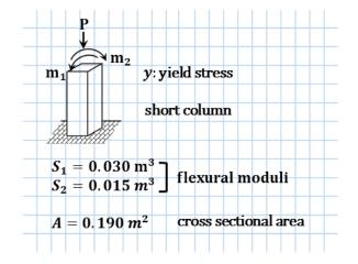
$\beta_{FORM} = 2.47$   $\mathbf{u}^* = \{1.21 \quad 0.699 \quad \theta.94 \text{ f}^T$   $\mathbf{x}^* = \{341 \quad 170 \quad 3223^T \quad 31.$   $\hat{\boldsymbol{a}} = \{0.491 \quad 0.283 \quad \theta.381$   $P_f \simeq \Phi(-\beta_{FORM}) = 0.00682$
