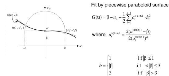
Merit: Insensitive to the noise in calculating  $g(\mathbf{x})$
