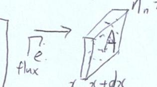
$$\Gamma(x+dx) = \Gamma(x) - \int(x) N_n A dx \frac{\sigma}{A}$$
