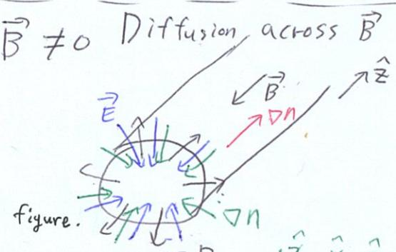
$$\begin{aligned} M &= \frac{e}{m\nu} = \frac{eB}{m\nu B} = \frac{w_c}{2B} \\ D &= \frac{kT}{m\nu} = \frac{eB kT}{m\nu B e} = \frac{w_c kT}{2eB} \\ \frac{E_y B}{B^2} &\downarrow \\ u_E & \text{exB drift} \end{aligned}$$
