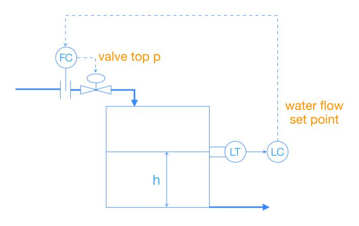
cascades the level controller to a water flow controller
