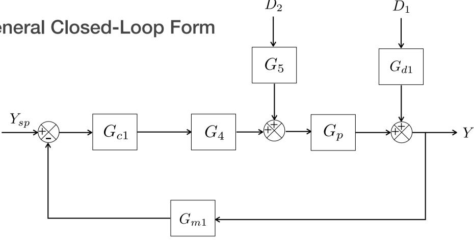
$$\frac{Y}{Y_{sp}} = \frac{G_{c1}G_4G_p}{1 + G_{c1}G_4G_pG_{m1}} = \frac{G_{c1}\frac{G_{c2}G_v}{1 + G_{c2}G_vG_{m2}}G_p}{1 + G_{c1}\frac{G_{c2}G_v}{1 + G_{c2}G_vG_{m2}}G_pG_{m1}}$$
