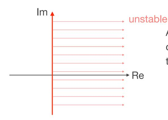
At the limits of instability, the closed-loop poles will be on the imaginary axis
