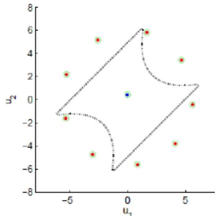
Complex failure domain by a series system (Waarts, 2000)
