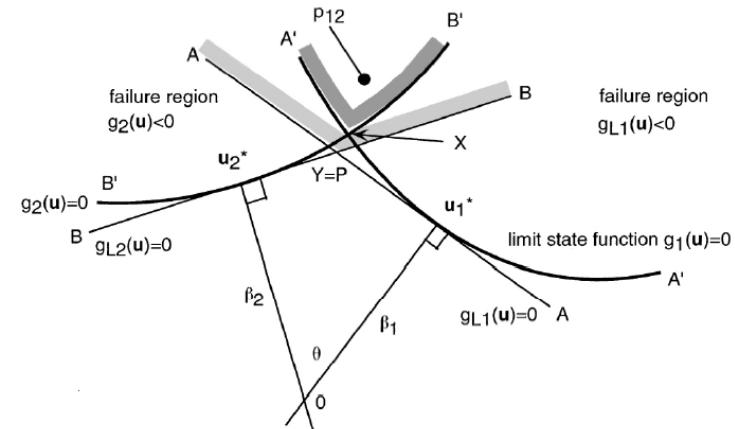
Parallel system problems and “joint design point” (Melchers & Ahammed, 2001)
