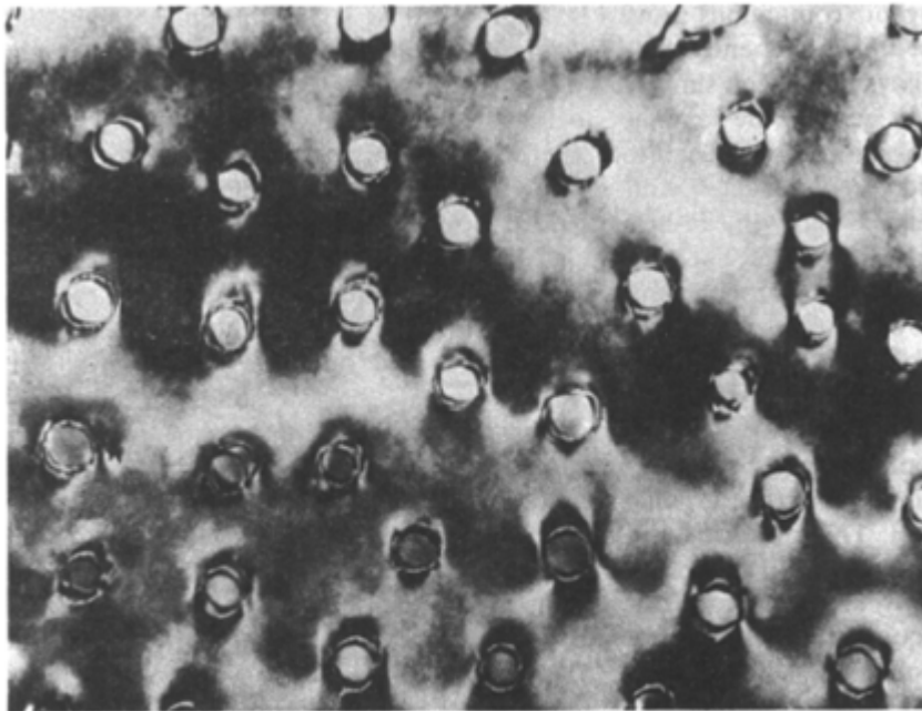
Fig. 4.30 Rod-like eutectic. \text{Al}_6\text{Fe} rods in Al matrix. Transverse section. Transmission electron micrograph ( x 70000).
