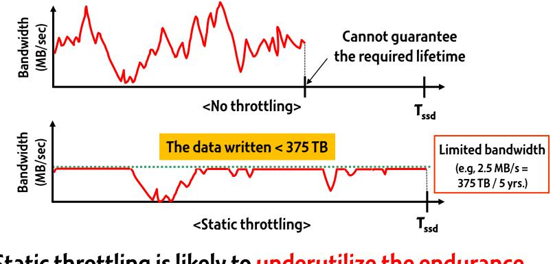
Static throttling is likely to underutilize the endurance of SSDs, incurring performance degradation
