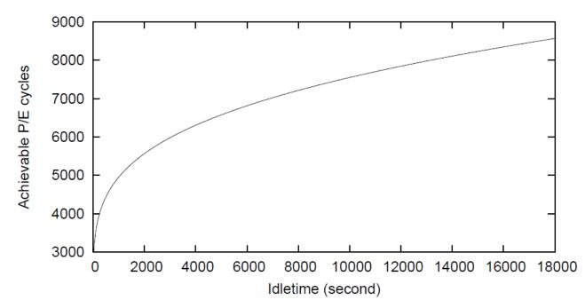
The endurance can be improved if the self-recovery is exploited in throttling write traffic...
