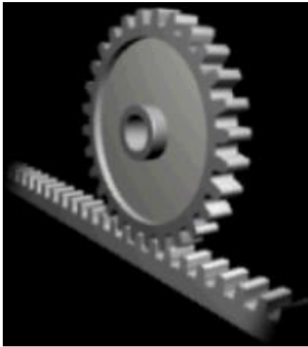
Rack and pinion (source:Wikipedia)
