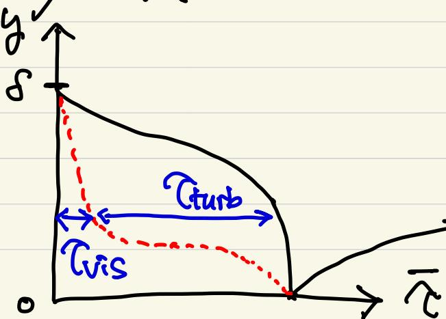
$$-\overline{\rho \bar{u}' \bar{v}'} = \mu_t \frac{\partial \bar{u}}{\partial y} \quad (\text{Prandtl})$$
