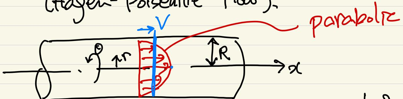
continuity eq:  $\frac{1}{r} \frac{\partial}{\partial r} (r v_r) + \frac{1}{r} \frac{\partial}{\partial \theta} v_\theta + \frac{\partial u}{\partial x} = 0$
