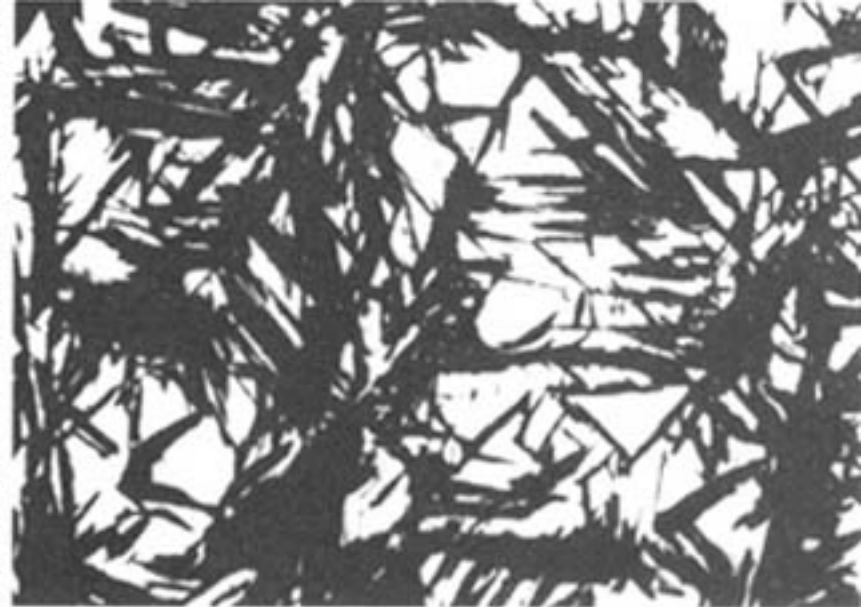
"Needle like" Structure of martensite
