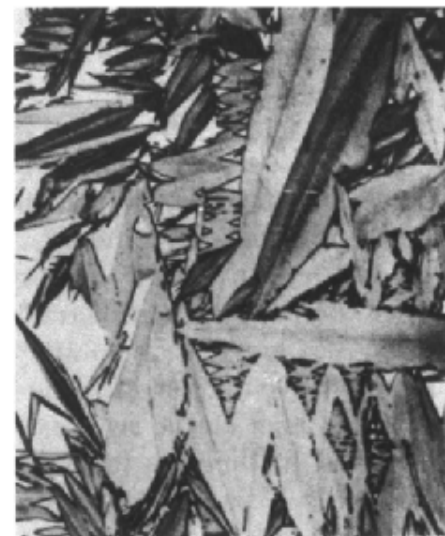
(e) Fe-Ni (plate, some isothermal growth)
