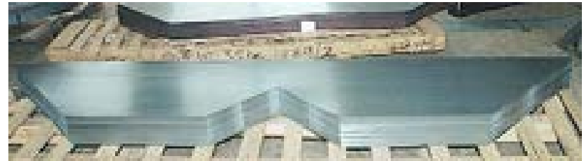
Stacked transformer core
