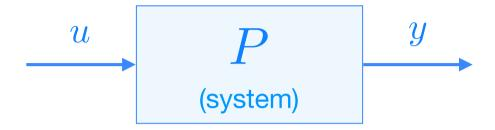
System can be seen as a mapping between input u and output y
