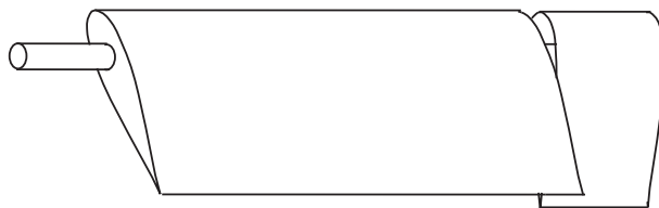
Figure 2.27: Excitation of outboard blade segment to generate oscillatory lift
