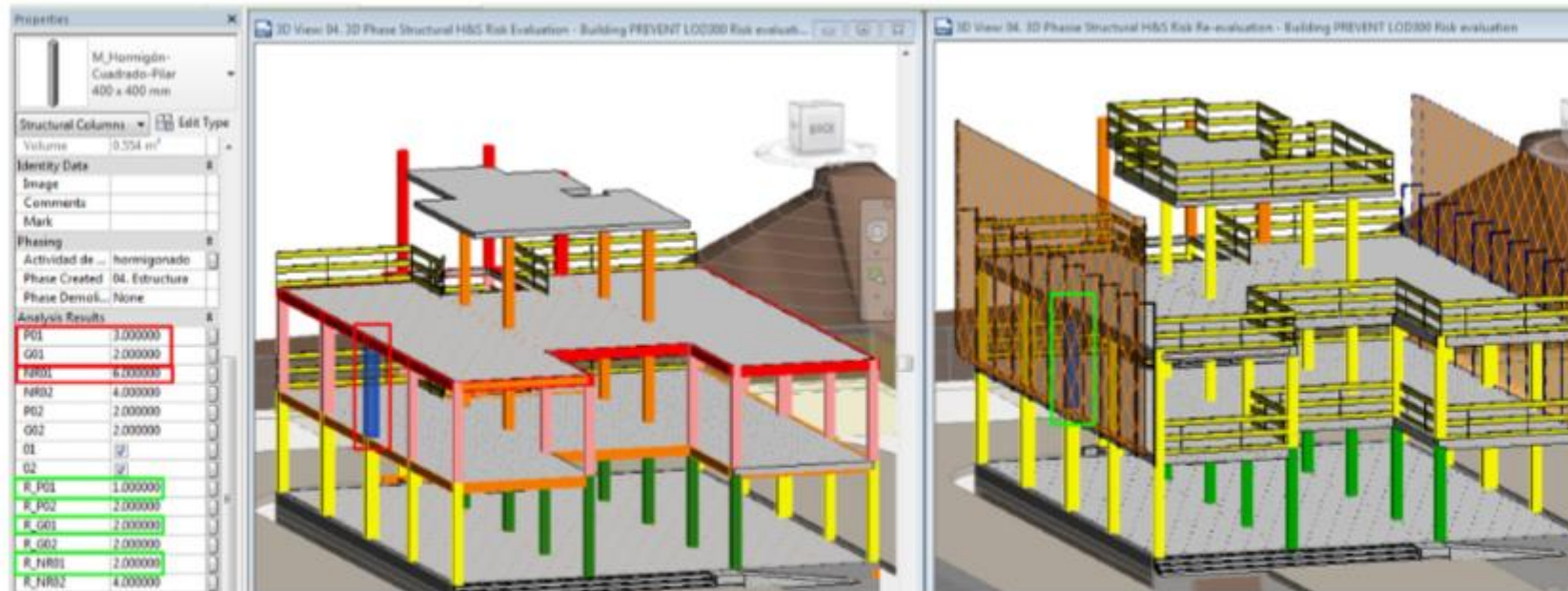
Fig. 9. Three-dimensional views for risk assessment 01 "People falling between different levels" (left) and after re-evaluation (right) with the pillars marked in colour based on the risk.
