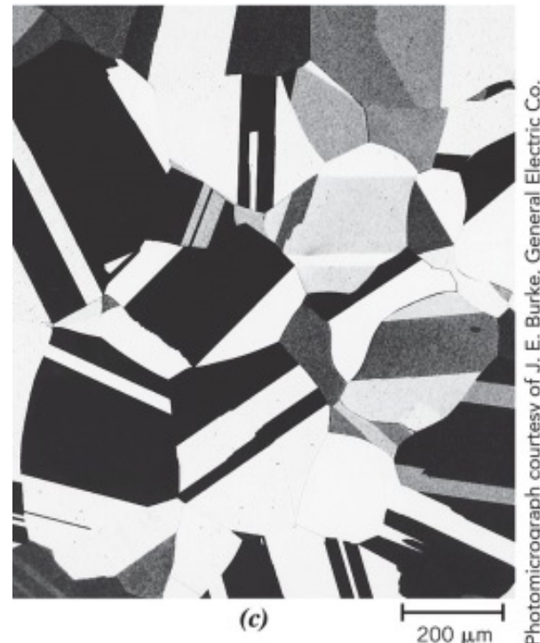
micrograph of Brass (Cu and Zn)
