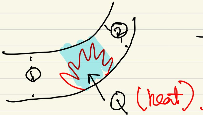
$$\Rightarrow \frac{P_1}{\rho} + \frac{1}{2} V_1^2 + g z_1 = \frac{P_2}{\rho} + \frac{1}{2} V_2^2 + g z_2 + \underbrace{W_s + W_f}_{\text{friction loss}} - \underbrace{W_q}_{\text{heat}}$$
