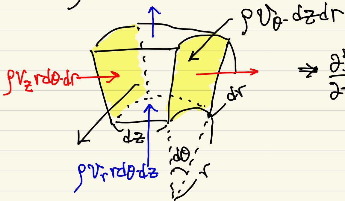
$$\Rightarrow \frac{\partial \rho}{\partial t} + \frac{1}{r} \frac{\partial}{\partial r} (r \rho V_r) + \frac{1}{r} \frac{\partial}{\partial \theta} (\rho V_\theta) + \frac{\partial}{\partial z} (\rho V_z) = 0.$$
