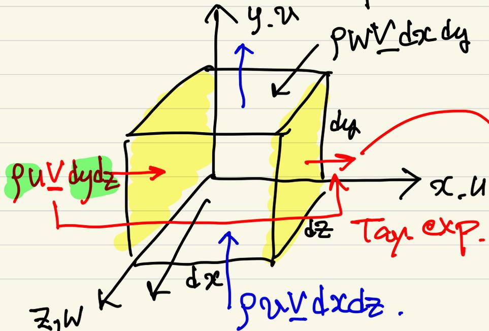
$$\sum \underline{F} = \frac{\partial}{\partial t} \int_{CV} \rho \underline{V} dV + \int_{CS} \rho \underline{V} (\underline{V}_n \cdot \underline{n}) dA$$
