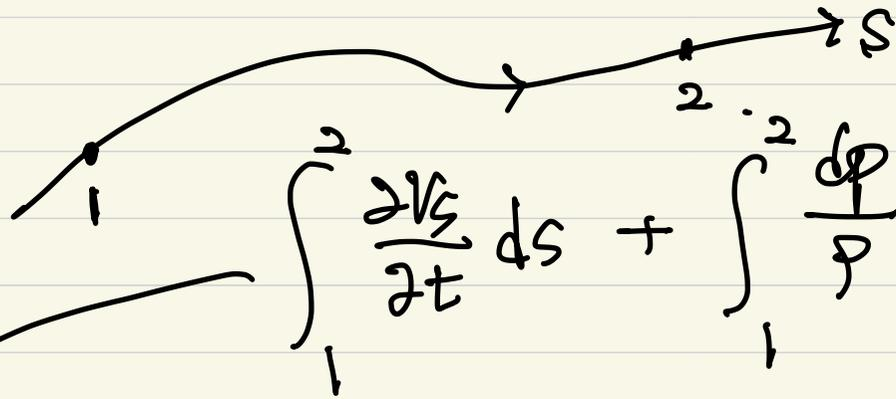
$$\int_1^2 \frac{\partial V_s}{\partial t} ds + \int_1^2 \frac{dp}{\rho} + \frac{1}{2} (V_2^2 - V_1^2) + g(z_2 - z_1) = 0$$
