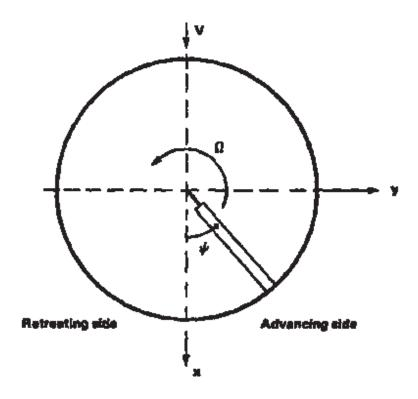
Typically, the value of  $\kappa_x$  is positive and the value of  $\kappa_y$  is negative. This means that the induced inflow is larger at the rear of the disk and on the retreating side. At higher velocities,
