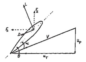
Quasisteady theory is used to obtain the aerodynamic forces. The  $u_p$  and  $u_T$  are flow velocity components. Forces per unit span are
