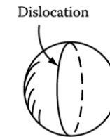
(c) Precipitate with dislocation
