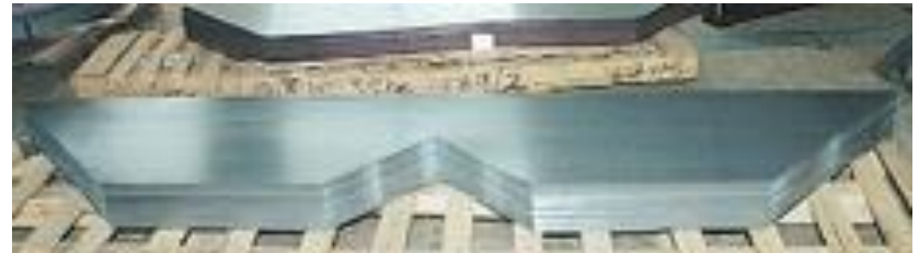
Stacked transformer core
