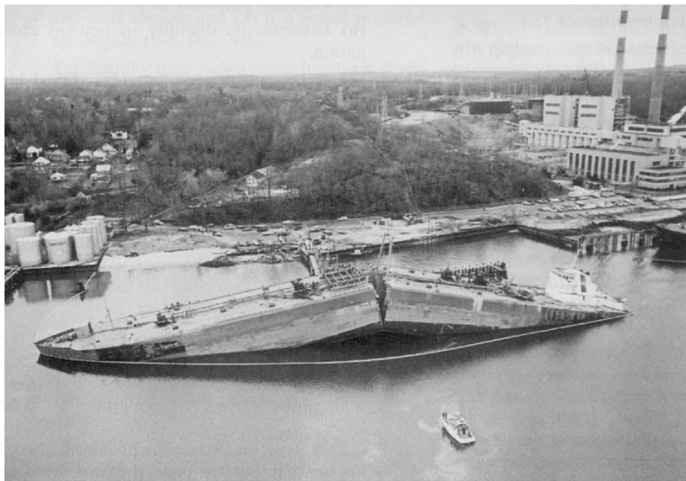
Oil tanker fractured in a brittle manner
