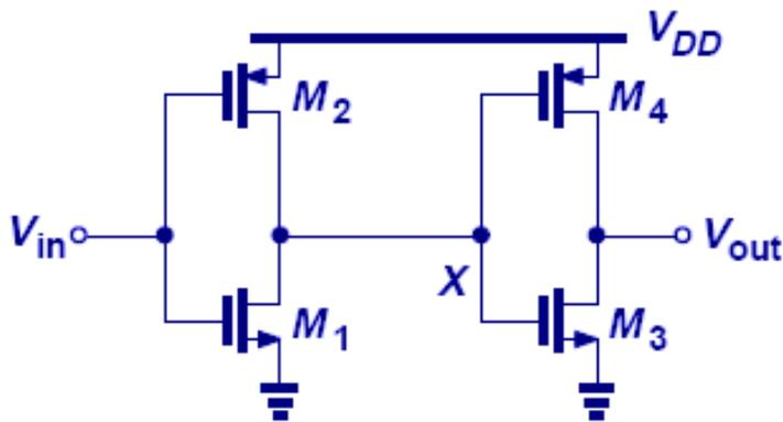
$$R_{on} = \frac{1}{\mu_n C_{ox} \left(\frac{W}{L}\right) (V_{DD} - V_{TH})}$$
