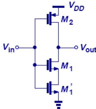
$$\begin{aligned} R_{on} &= R_{on1} + R_{on1'} \\ &= \frac{1}{\mu_n C_{ox} \left(\frac{W}{L}\right)_1 (V_{DD} - V_{TH1})} + \frac{1}{\mu_n C_{ox} \left(\frac{W}{L}\right)'_1 (V_{DD} - V'_{TH1})} \\ &= 2R_{on1} \end{aligned}$$
