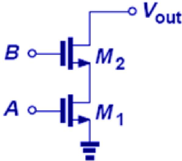
➤ When both  $A$  and  $B$  are high, the output is low.
