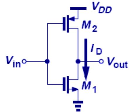
Region 1:  $M_1$  is off and  $M_2$  is on.  $V_{out} = V_{DD}$ .
