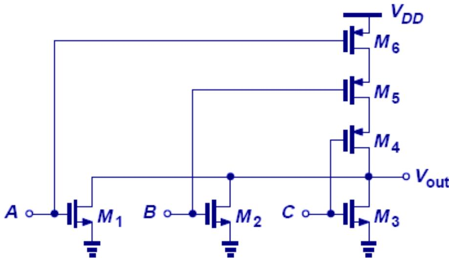
$$V_{out} = \overline{A + B + C}$$
