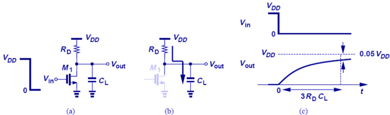
$$V_{out}(0^-) = \frac{V_{DD}}{1 + \mu_n C_{ox} \frac{W}{L} R_D (V_{DD} - V_{TH})} \quad V_{out}(t) = V_{out}(0^-) + [V_{DD} - V_{out}(0^-)] \left( 1 - \exp \frac{-t}{R_D C_L} \right), t > 0$$
