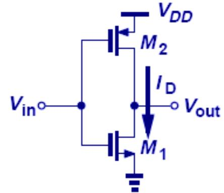
Region 4: Similar to Region 2. *M*<sub>1</sub> is in triode region and *M*<sub>2</sub> is in saturation. Valid only when  $V_{out} \leq V_{in} - V_{TH1}$ .
