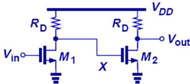
$$\begin{aligned} \text{Assuming } C_X &\approx WLC_{ox} \text{ and } R_D = 19R_{on1}, \\ \tau = R_D C_X &= \frac{19}{\mu_n C_{ox} \frac{W}{L} (V_{DD} - V_{TH})} \cdot WLC_{ox} \\ &= \frac{19L^2}{\mu_n (V_{DD} - V_{TH})} \end{aligned}$$
