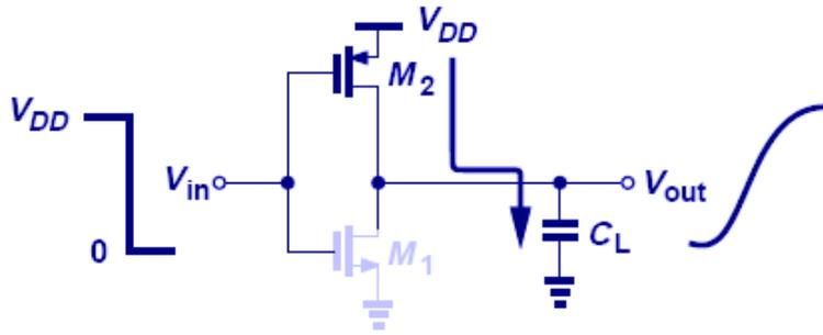
$$P_{Dissipation\_PMOS} = \frac{1}{2} C_L V_{DD}^2 f_{in}$$
