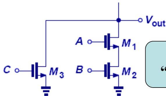
C is in “parallel” with the “series” combination of A and B
