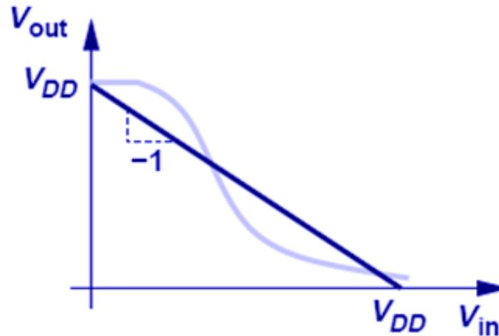
➤ **The transition region at the input spans a range narrower than 0 to  $V_{DD}$ .**
