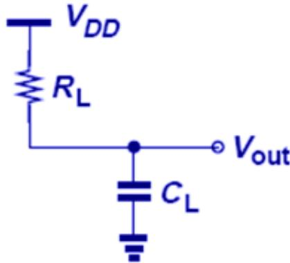
$$E_{\text{stored}} = \frac{1}{2} C_L V_{DD}^2$$
