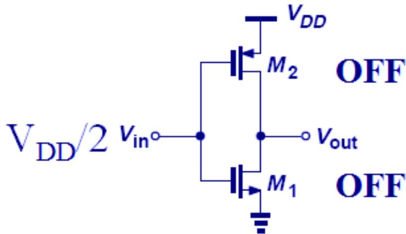
If  $V_{DD} < V_{TH1} + |V_{TH2}| = 2 V_{TH}$ ,
