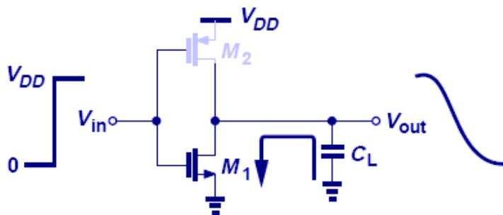
$$P_{Dissipation\_NMOS} = \frac{1}{2} C_L V_{DD}^2 f_{in}$$
