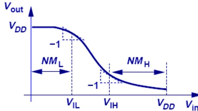
1. Using the small-signal gain :  $g_m R_D = \mu_n C_{ox} \frac{W}{L} (V_{IL} - V_{TH}) R_D = 1$
