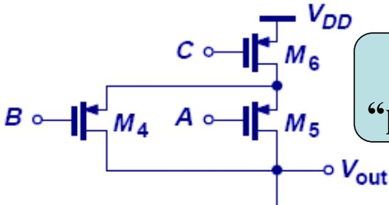
C is in “series” with the “parallel” combination of A and B
