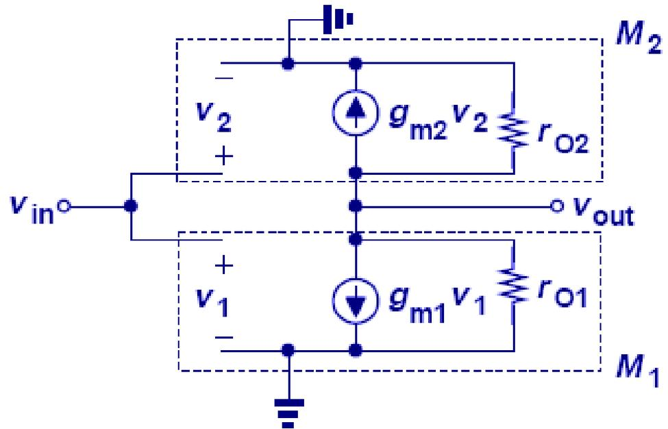
$$\frac{v_{out}}{v_{in}} = -(g_{m1} + g_{m2})(r_{O1} \parallel r_{O2})$$
