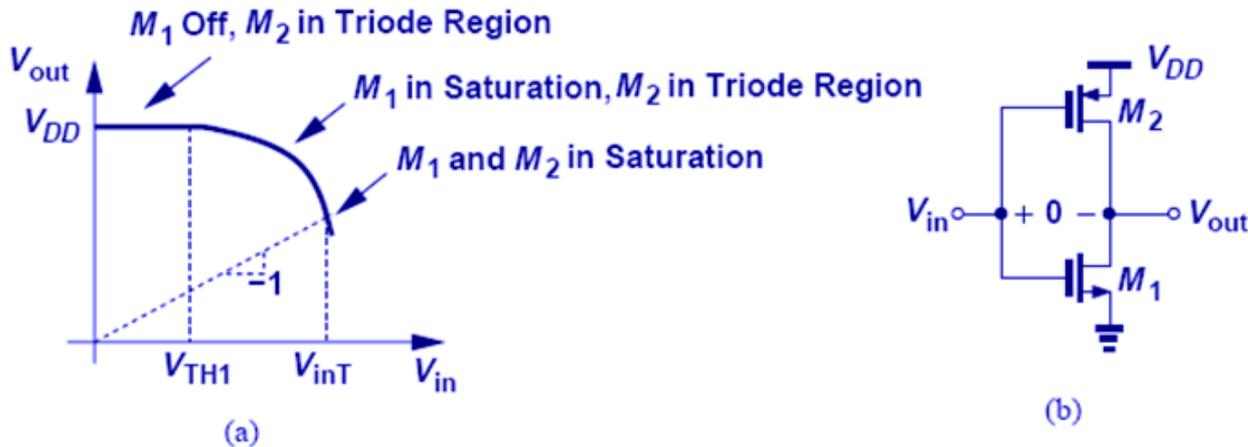
$$\mu_n C_{ox} \left( \frac{W}{L} \right)_1 \left( \frac{V_{DD}}{2} - V_{TH1} \right)^2 \left( 1 + \lambda_1 \frac{V_{DD}}{2} \right) = \mu_p C_{ox} \left( \frac{W}{L} \right)_2 \left( \frac{V_{DD}}{2} - |V_{TH2}| \right)^2 \left( 1 + \lambda_2 \frac{V_{DD}}{2} \right)$$
