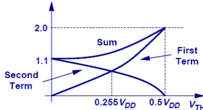
$$T_{PLH/HL} = \frac{C_L}{\mu_{p/n} C_{ox} \left(\frac{W}{L}\right)_{2/1} [V_{DD} - |V_{TH2/1}|]} \left[ \frac{2|V_{TH2/1}|}{V_{DD} - V_{TH2/1}} + \ln \left( 3 - 4 \frac{V_{TH2/1}}{V_{DD}} \right) \right]$$
