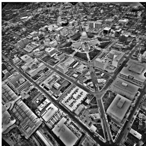
Figure 1-6. Low oblique photograph of Madison, Wisconsin (note that the horizon is not shown)
