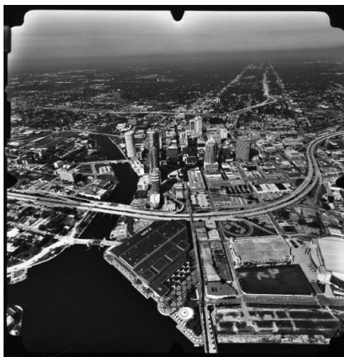
Figure 1-7. High oblique photograph of Tampa, Florida (note that the horizon shows on the photograph)
