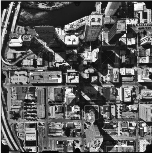
Figure 6-7. Vertical photograph of Tampa, Florida, illustrating relief displacements. (Courtesy US Imaging, Inc.)
