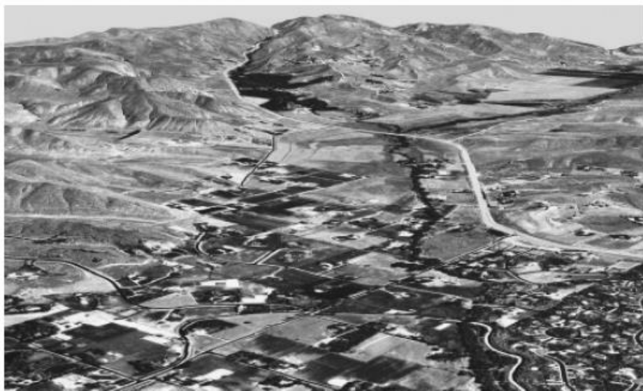
Figure 13-9. Three-dimensional pictorial view of terrain obtained by combining a DEM and orthophoto.
