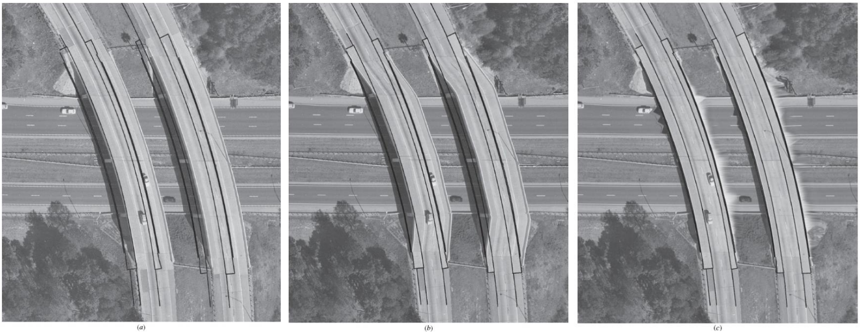
Figure 13-8. Effect of DEM accuracy on orthorectification.
