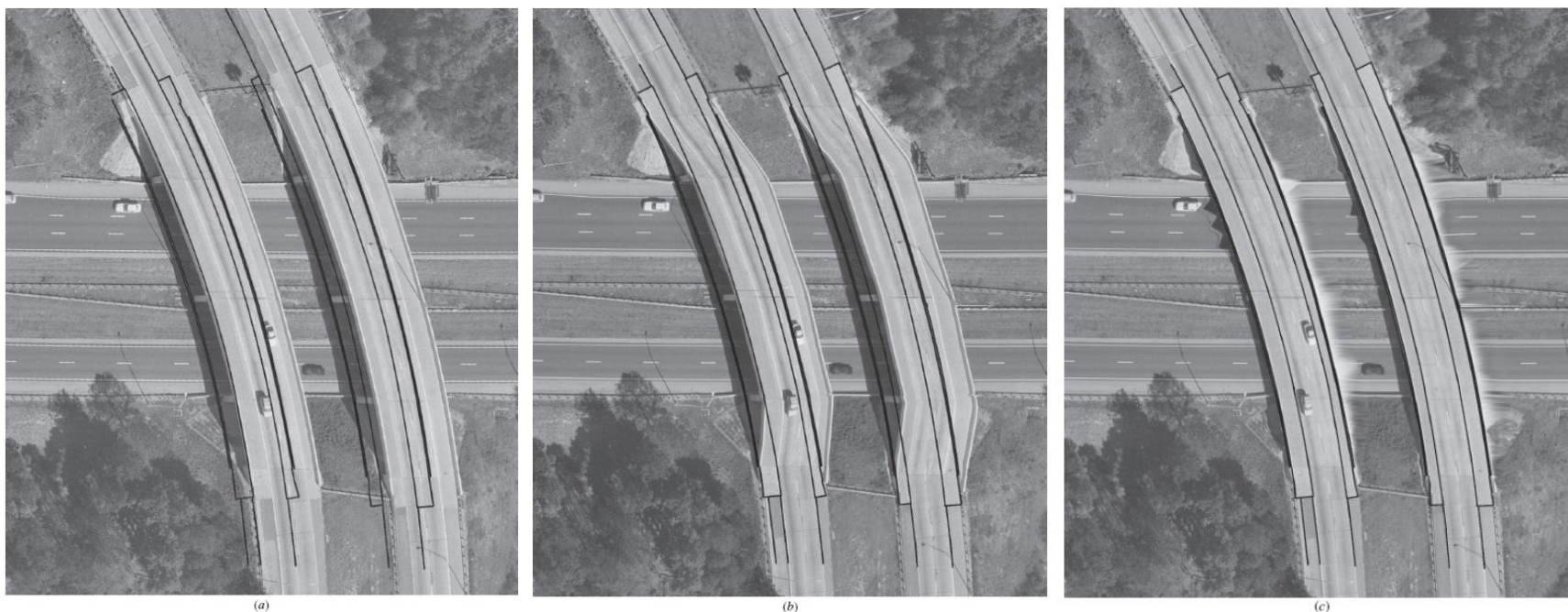
Figure 13–8. Effect of DEM accuracy on orthorectification.
