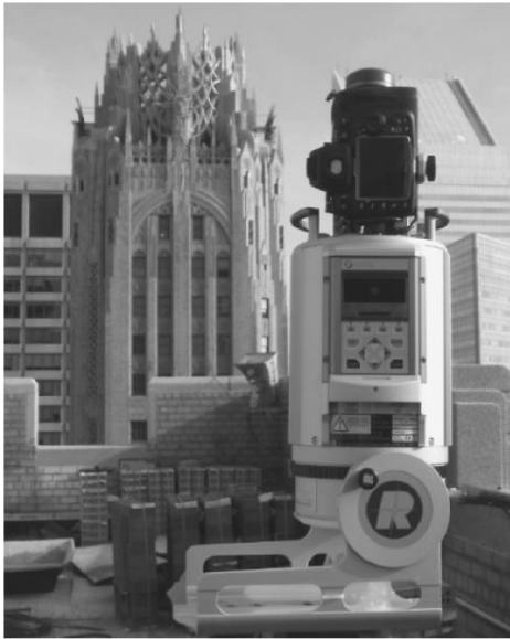
Figure 14-5. RIEGL VZ400 terrestrial laser scanner. (Courtesy of RIEGL USA, Inc.; http://www.rieglusa.com .)
