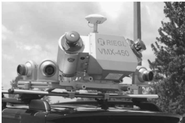
Figure 14-6. RIEGL VMX450 mobile laser mapping system. (Courtesy of RIEGL USA, Inc.; http://www.rieglusa.com .)
