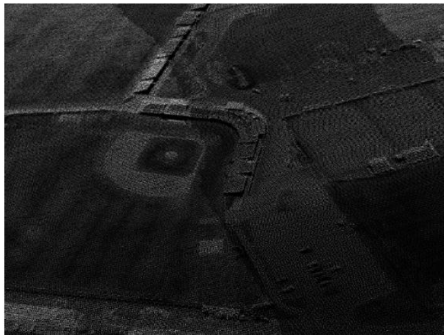
Figure 14-1. Combined aerial photography and laser scan data. (Image courtesy of Optech)
