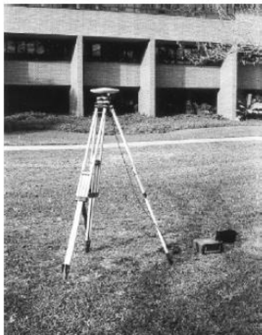
Figure 16–8. GPS receiver with antenna mounted on a tripod. (Courtesy University of Florida.)
