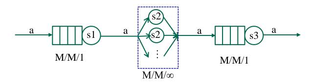
$$- n_1 = \frac{a \times s1}{1 - a \times s1}, \quad T_1 = \frac{s1}{1 - a \times s1}, \qquad T_2 = s2, \qquad n_3 = \frac{a \times s3}{1 - a \times s3}, \quad T_3 = \frac{s3}{1 - a \times s3}$$
