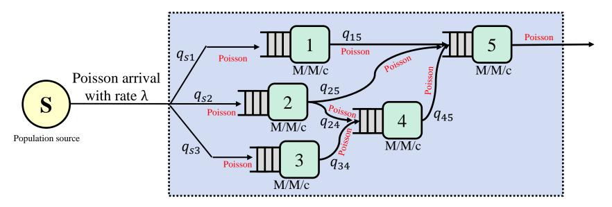
Each device is modeled as M/M/c, being independent of each other.
